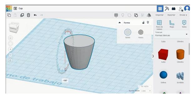
7. Copy the paraboloid shape and size it to 38x38x34 mm, then we put in the center of the original shape. We will use it later to empty the core.
