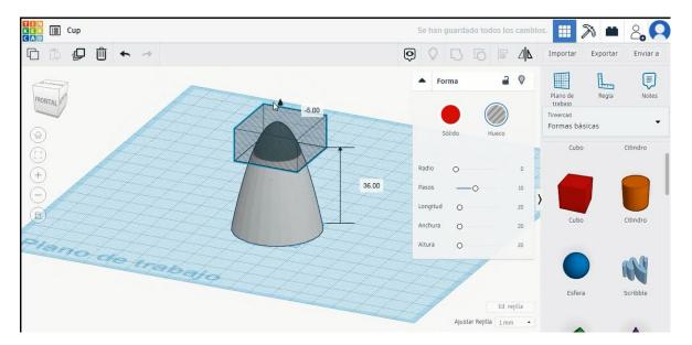
5. Pressing Shift and selecting the paraboloid and the cube, select group
