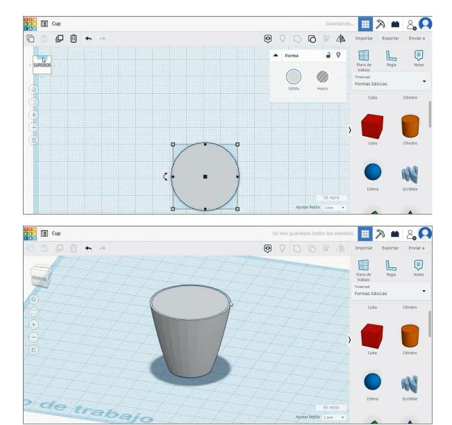
8. To create the handle, choose the torus in color mode and rotate it to put in the right top side of the cup. Then, pressing shif and selecting the cup and the torus press group to merge both.
