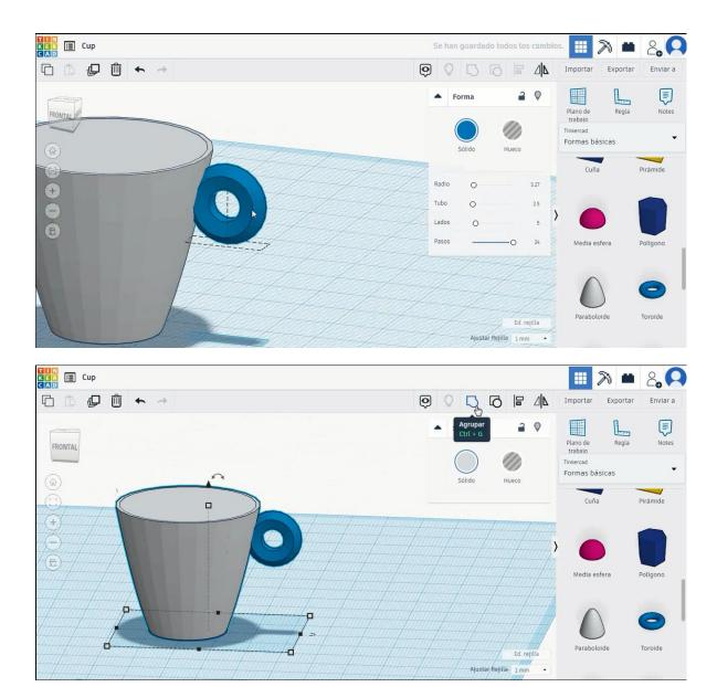
9. Select the smaller paraboloid that we have created before and choose hole mode. Select both entities pressing shift key and then select group to empty the core.
